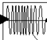
Curve below is magnified to show how the FM-voice controls the timing of the transmitter's pulses.
