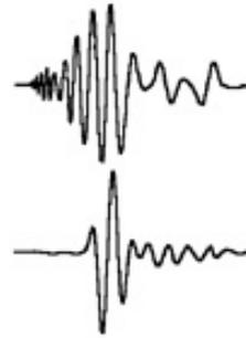
The key to Patriot's Radar system is its ability to transmit and receive pulses barely longer than single cycles at the transmit frequency. The first waveform shown here is a pulse generated by an earlier Patriot Design, based on "off the shelf" antenna technology. The waveform on the bottom was produced and received by Patriot's current Design.
