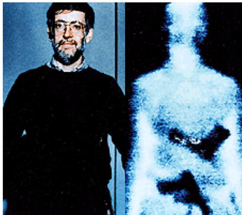
Millimeter-wave camera picks up both metallic and plastic concealed handguns.
