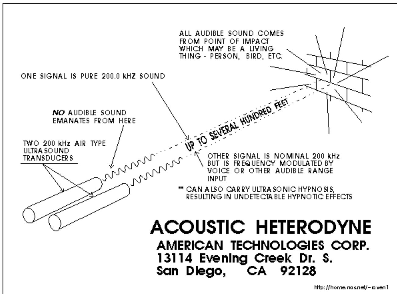
Illustration showing the principle of an ultrasound projection system capable of true ventriloquism at a distance, by American Technologies Corporation (licensor), Akai Japan (licensee)
