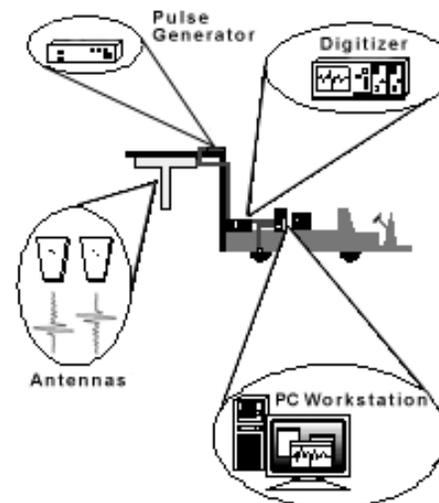
...is a diagram of the demonstration system. A pulse generator is used to drive the transmit antenna. The pulse is a positive spike going up to 100V then falling back to ground in one and a half nanoseconds corresponding to a pulse transmit frequency of 750 MHz.
