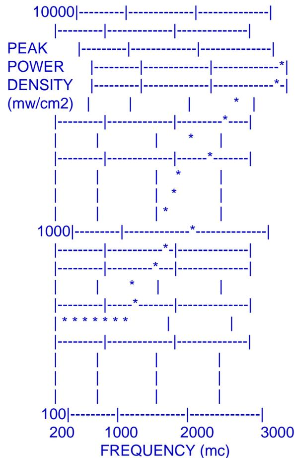
FIG. 5. Microwave power distribution in a forehead model neglecting resonance effects and considering only first reflections (from Nieset et al. (5), modified).
