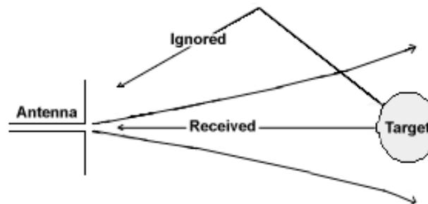
Interference with other sources and receivers is further reduced by using directional antennas. The antenna design shown is highly directional.
